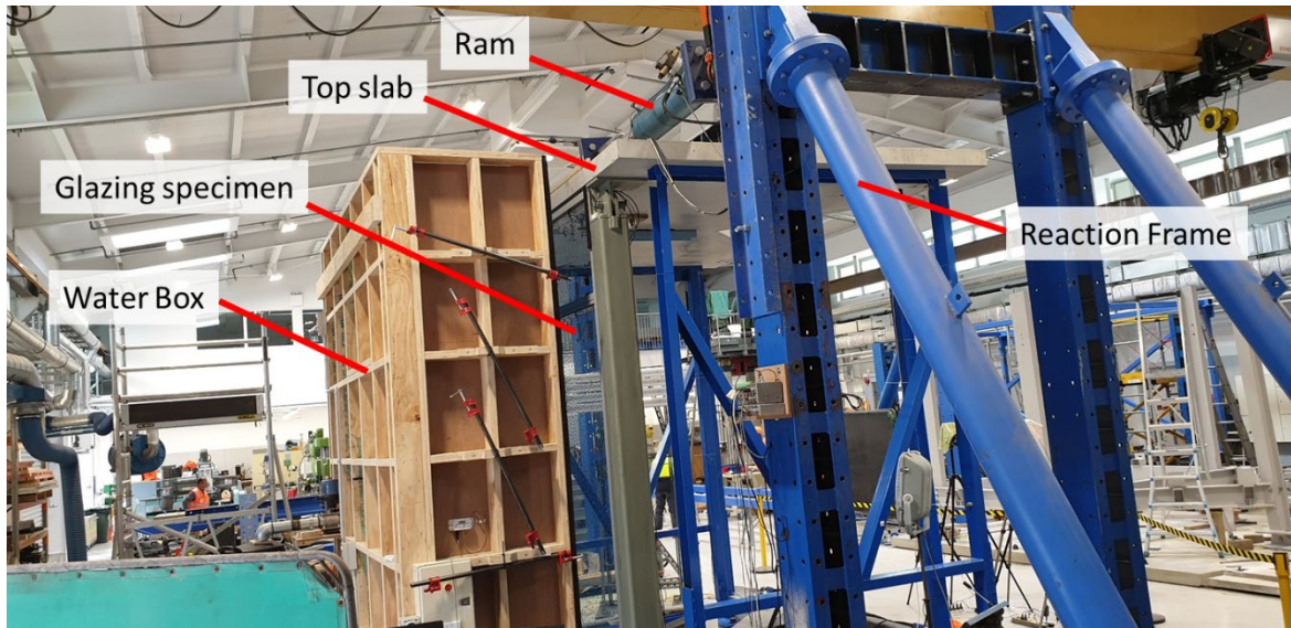
Figure 3. Photo of water box, actuator, reaction frame and ram.
