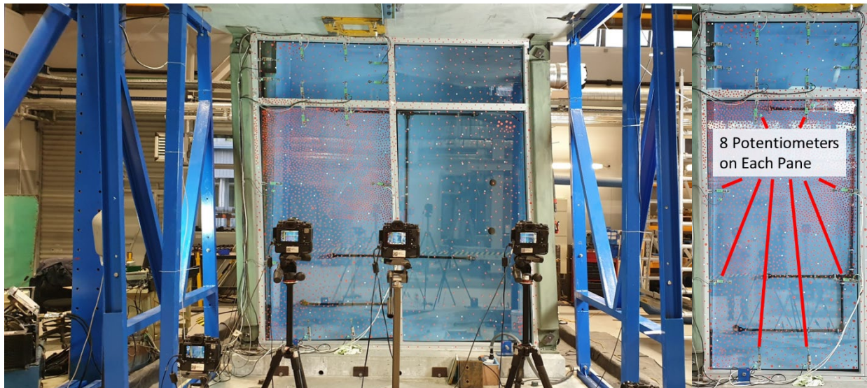
Figure 8. Photo showing glazing specimen and instrumentation used in the experimental testing, cameras and red dots used for particle-tracking (left) and potentiometers used to monitor displacements of panes relative to framing (right).
