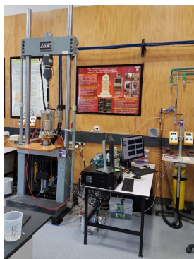
Figure 2: Cyclic triaxial test set-up
