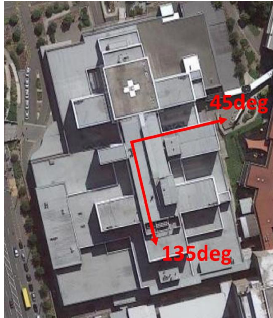
Figure 5: Plan view of the Wellington Hospital Building showing the principle component directions (Source: Google Maps)
