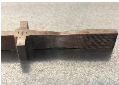
Loaded plate failure in samples made by partial penetration welds
