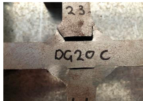
Weld failure in some samples made by fillet welds
