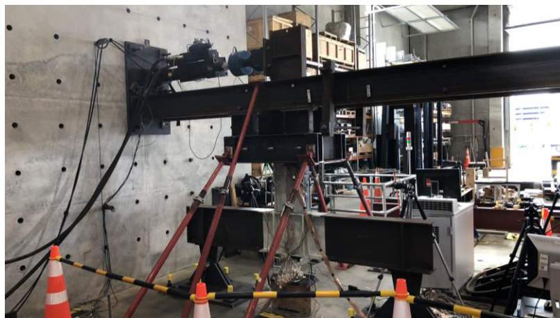
Figure 2: Test setup based on the SAC protocol
