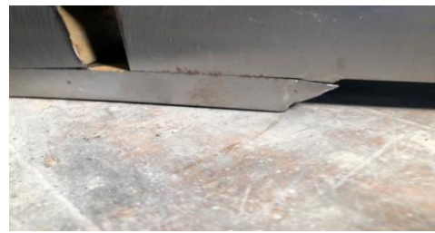
Transverse shear weld specimens
