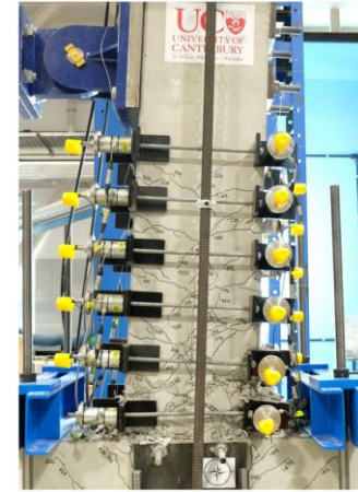
Figure 5: a) Hysteretic response of columns C5 and C6; b) Column C5 at a drift ratio of 5.5%; c) Column C6 at a drift ratio of 5.5%
