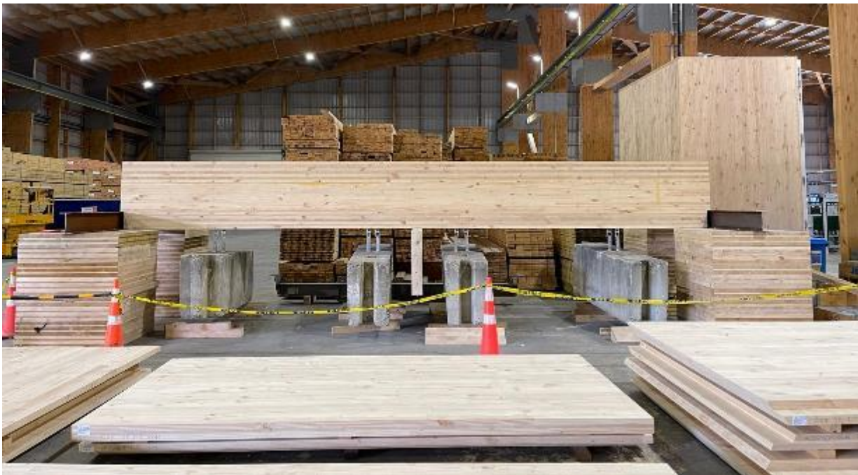
Figure 4: Test Beam Setup
